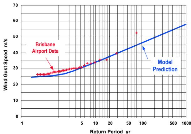
**Figure 4 - Modelled versus Measured Wind Gusts at Brisbane Airport**
